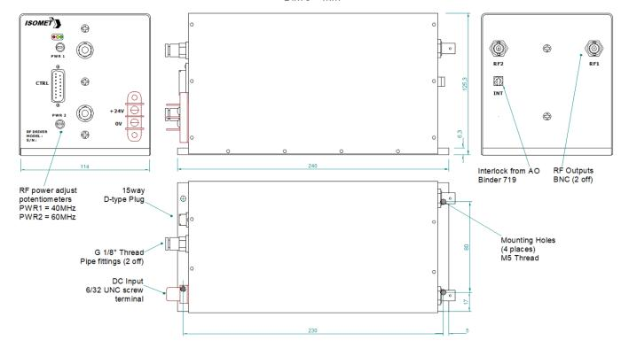
Heatsink in contact with coolant water. Default aluminium. See BR option. Water-coolant fittings supplied are suitable for 8mm OD / 6mm ID pipe.
